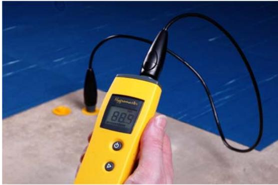
As an alternative to surface ERH readings, Hygrosticks can be put into humidity sleeves that are placed into holes drilled into the slab.
