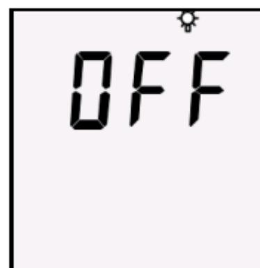
If the unit detects no key press for 2 seconds in the Setting screen, it moves to the next setting.
